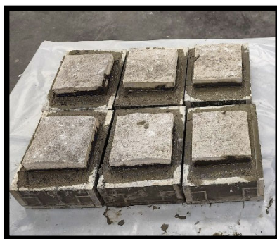
Shear blocks molded per C482 [L] and sample under test in Universal Testing Machine (UTM) [R]
