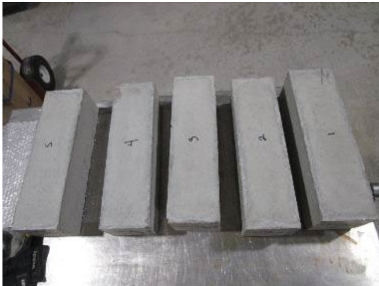
Photo No. 2 ASTM C1670 / ASTM C666 Specimens Before Exposure
